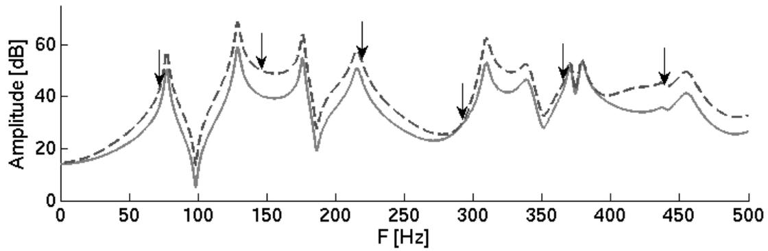
(a) Soundboard FRF without (—) and with (- - -) combined control for the first control configuration.
