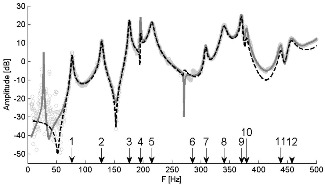
Figure 6: FRF ( $\circ$ ), modal reconstruction ( $—$ ) and state space model ( $- - -$ ). Arrows indicate the modes' number.
