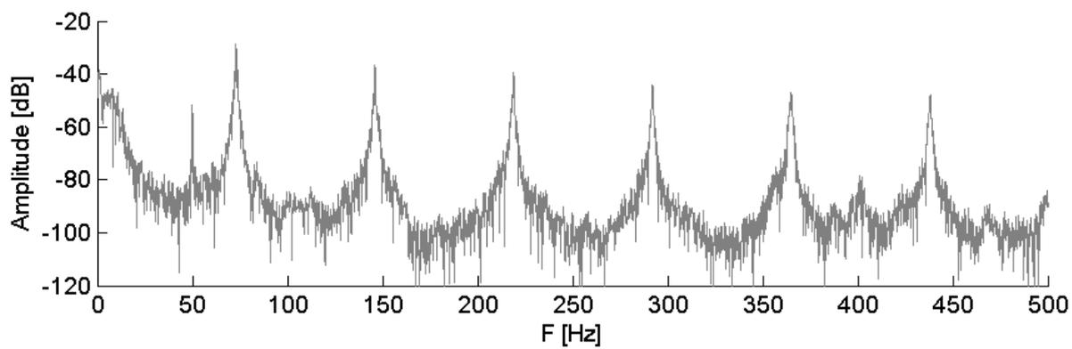
Figure 5: Fourier transform of the string signal whose fundamental frequency is approximately set to 75 Hz.
