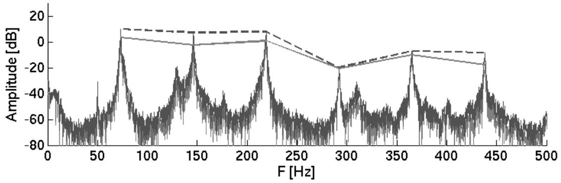
(a) Fourier transform shape of the measured signal without (—) and with (- - -) combined control for the first configuration.
