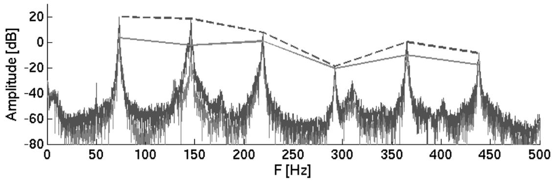
(b) Fourier transform shape of the measured signal without (—) and with (- - -) combined control for the second configuration.
