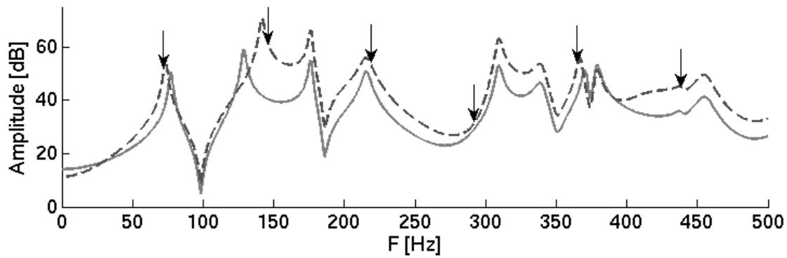
(b) Soundboard FRF without (—) and with (- - -) combined control for the second control configuration.
