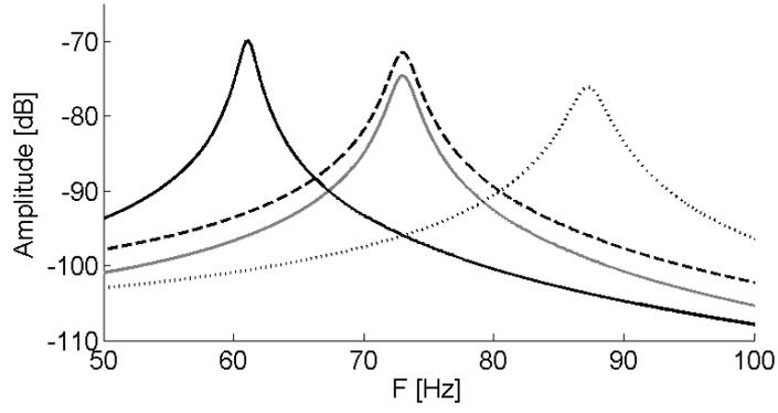
Figure 3: Amplitude of one mode without (—) and with (---) combined control. Results obtained with  $\mathbf{K}_2 = \mathbf{0}_{1,2n}$  (—) and  $\mathbf{K}_1 = \mathbf{0}_{1,2n}$  (.....).
