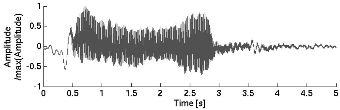
(a) String's force signal used as disturbance on the numerical soundboard model applied to the bridge location.
